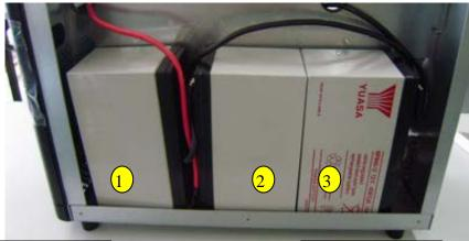
3. Put the three batteries in order as shown in chart. Hint: Install the left one and keep battery terminal heading the bottom. Then, install the middle one and keep battery terminal heading upwards. At least, install the right one and keep battery terminal heading upwards.
