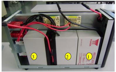
7. Put the three batteries in order as shown in chart. Hint: Install the left one and keep battery terminal heading the bottom. Then, install the middle one and keep battery terminal heading upwards. At least, install the right one and keep battery terminal heading upwards.
