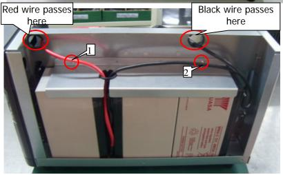
4. Put grommet inside the hole of battery divider and allow red and black wire passing through the hole. Screw tightly the battery divider with screw nuts. (as shown in 1, 2 areas)
