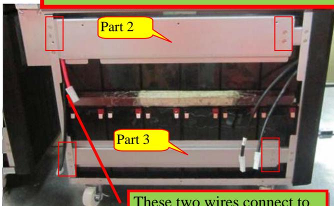
3. Screw up the Part2 & Part3 on the case by using 8 flat head screws;
