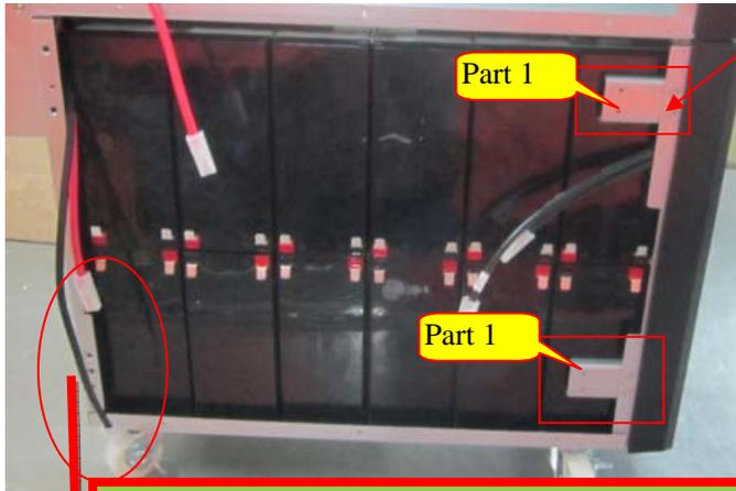
1. Put 12 batteries in the left side of bottom case. (**CAUTION: Keep the electrode away of the case;**)
