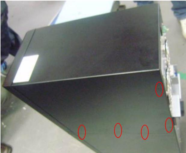
Screw up the top cover of the battery bank;
