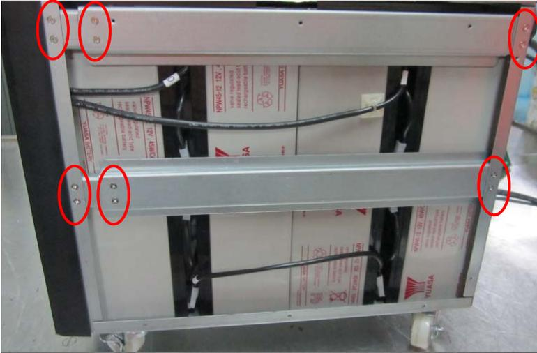
Screw up the guardrail like the picture on the left;
