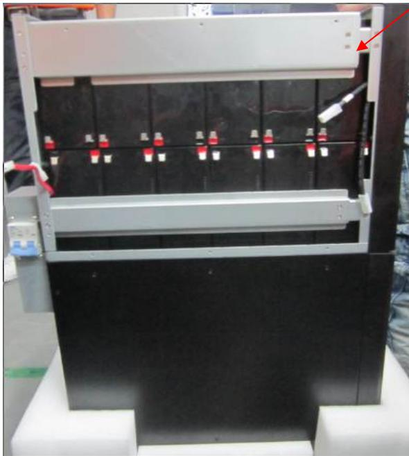
1. Put 12 batteries in the left side of the top case. (just like the bottom case)
