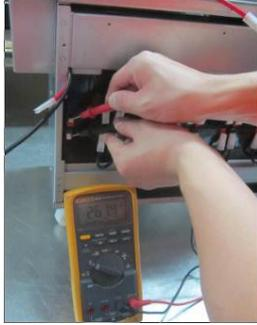
Check the voltage before connect the ANEN connector;
