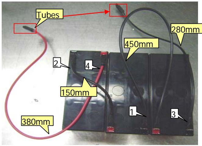
1. As shown, please use three batteries (12V/7Ah or 12V/9Ah) and check the date code (it's necessary to use batteries with same date code in a UPS unit). Serial connect batteries with three black wires in 450, 280, 150 mm length. Slip the end of black wire with 280mm length into the tube.
