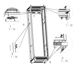
I&IV steps, use M8\*12 screw and nuts fix top andbottom cover, II step use M4\*8 self Tapping Screws fixed Fan tray on the top Frame. Step III, use M4\*8 Self Tapping Screws fixed doorstops on the four side of Frames.
