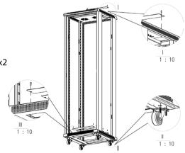
I & III, step, use M4\*8 Self-Tapping Screw to fixe entry panel on top and bottom Cover. II step use M5\*8 Self--Tapping Screw to install the castors.
