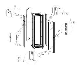
I to IV Steps Install Locks and Doors. Krok I do IV zamontuj drzwi i zamki.
