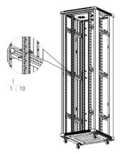
I Step, Use M6\*12 Screw to fix the connect bar to the frame. And then use M6\*12 Screw to fixe the mounting elements to the connect bars.
