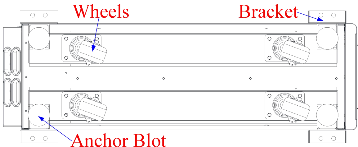
Fig.3-1 Supporting structure (Bottom view)
