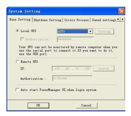
This particular window is used to select monitoring modes and associated with them options for UPS monitoring.
