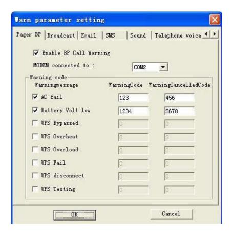
"Warning message", "WarningCode" and "CancelWarningCode" boxes are defined by the users. For example, the following "AC fail" message can be set along with "123" warning code and "456" alarm cancel code. At the time of the power failure, the end users will receive a "123" alarm message on their Pagers.
