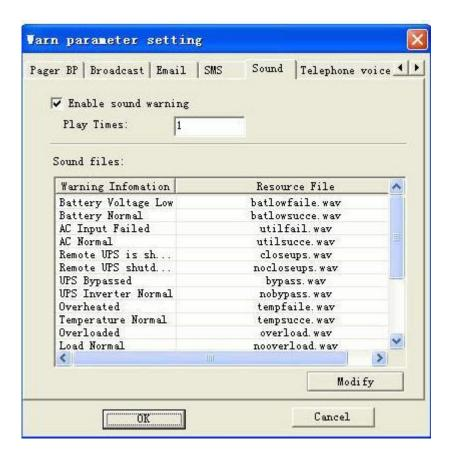
In the event of actual UPS status change, the software will send a sound alarm (signal) X times according to the individual needs.
