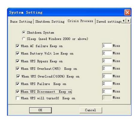
When this particular crisis management operation is enabled and its options correctly configured, the software will shut down the system during, above displayed, critical UPS situations, in a period of time selected by the users.
