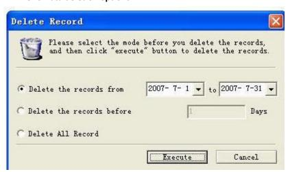
Data deletion feature of UPS history data has filter functions; therefore, users can delete events using options like:
