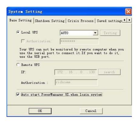
After selecting the desired options for the main interface, a confirmation window, like the one displayed below, will appear (Please note, that selecting the Powermanager II auto-start option, the software will launch along with system startup, so the following window will not be displayed.):
