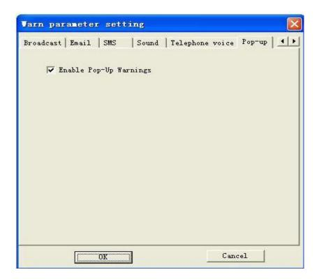
In the event of actual UPS status change, the software will display a pop up warning window. Pressing the "Close" button will close this window, which will reappear, only when the next alarm situation occurs.
