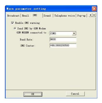
Then user has to select appropriate communication port, to which GSM modem is connected "GSM Modem connected to" and set the "Baud rate" according to actual usage. The last field left to fill in, is "SMS center". Sample SMS Center value is e.g.: +8613800200500.
