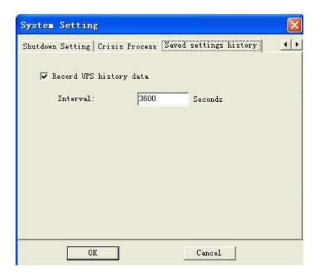
By enabling option "Save UPS history data", the software will record UPS history data according to the interval, specified by the users. (If the is no need for such feature, it is recommended to set the value of "Interval" equal or longer than 1 hour).
