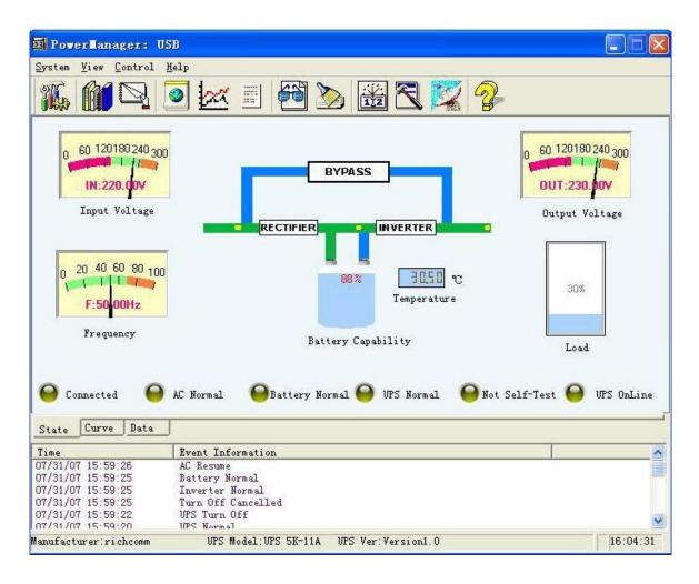
Using this chart, user can quickly check the following UPS status information: "Input Voltage", "Output Voltage", "Frequency", "Battery Capacity", "UPS Temperature" and "UPS Load".
