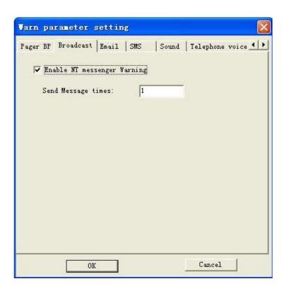
After pressing the "**OK**" button, in the event of UPS status change, the software will send a notification message X times according to the individual needs.
