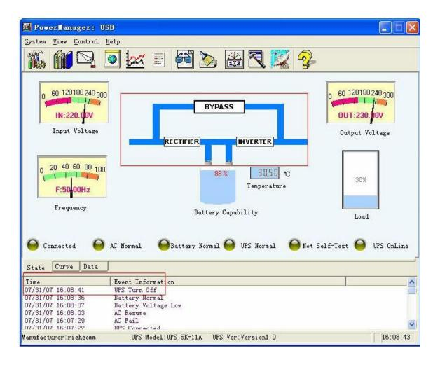
5. "UPS Fault" (error): Status line of the UPS has visibly changed, indicator "UPS failure" is glowing red and software is displaying brief information, regarding this particular, critical UPS event.
