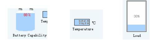
Further indicators illustrate the UPS battery capacity, which is at 88%, while the device temperature equals 30.50°C with the load level of 30%.
