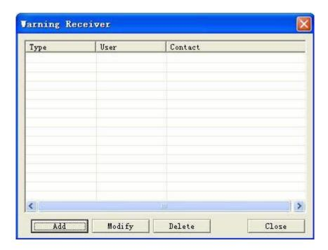
To properly add a recipient of Email notifications, the "Add" button must be first pressed. Users can also edit the previously added data of alarm message recipients, using the "Modify" button or simply delete the data, using the "Delete" button.
