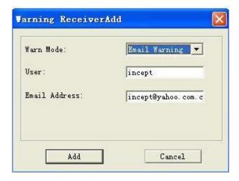
In the next step, user has to choose "Email alert" from the "Warning mode" field and fill in the remaining "User" and "Email Address" boxes. After all fields have been filled in properly, and the "Add" button is pressed, the email notification recipient will be successfully added.
