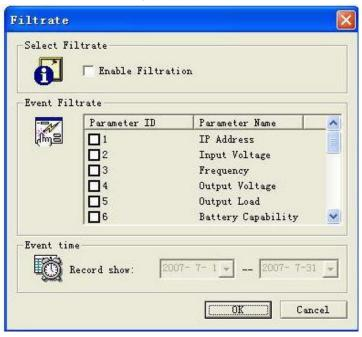
Feature, displayed above allows the users to sort the scope of UPS parameter data, using their "Parameter Name", as well as the time period, during particular events were recorded. Ticking the "Enable filter" option, then selecting specific filter scope "Event filter" and finally, pressing the "OK" button, will result in software, sorting the historic parameter data according to the user-selected guidelines.
