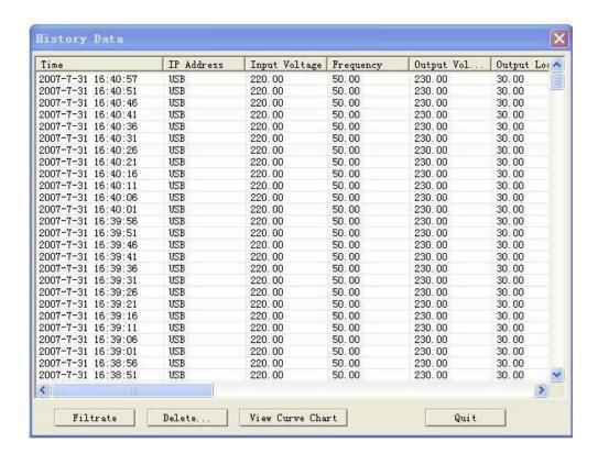
Displayed above, interface window contains information, how, during the user-specified periods of time, fluctuated values of parameters such as: Input Voltage, Output Voltage, Frequency, Load Output, etc.
