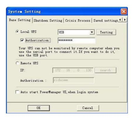
Choosing the "COM" options, the software will only search for active communications between the COM ports and the UPS. Users must select the correct COM port, otherwise the device(s) will not communicate with software properly.
