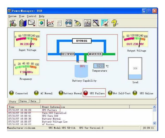
**6.** "UPS Test": Status line of the UPS has visibly changed, indicator "UPS Test" is glowing red and software is displaying brief information, regarding this particular, critical UPS event.
