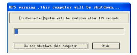
After the 2-minute countdown elapses, the system will shut down and go into sleep mode. Pressing "**Do not Shutdown this computer**" button will cancel the sleep mode from being enabled. Pressing "**Hide**" button will cause the countdown window to be hidden, while the PC will automatically go into sleep mode in 2 minutes.
