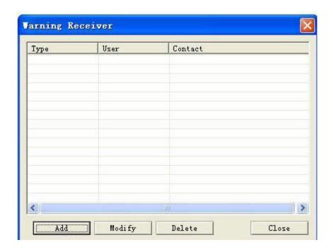
To properly add a recipient of Pager notifications, the "Add" button must be first pressed. Users can also edit the previously added data of alarm message recipients, using the "Modify" button or simply delete the data, using the "Delete" button.
