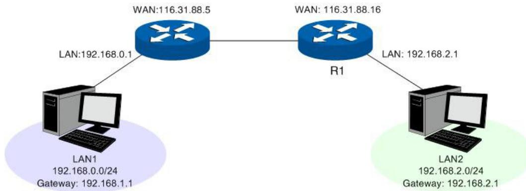
If the LAN port of TL-ER604W ( with Non-NAT or Classic system mode ) is connected to LAN1 with subnet of 192.168.0.0/24, while the LAN port of another Router R1 is connected to LAN2 with network of 192.168.2.0/24. Meanwhile, the WAN ports of the two routers are interconnected and within the same network. Now a host under TL-ER604W and within network of LAN1 desires to communicate with the host within network of LAN2.
